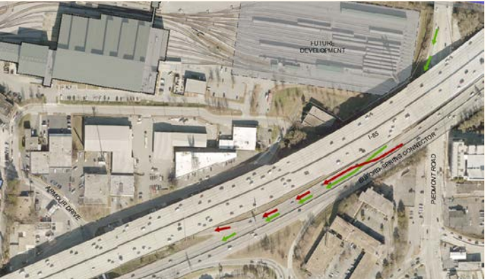
FIGURE 23. The existing weave configuration on Buford Highway. On-ramp traffic, shown in green, enters using the Piedmont ramp. Off-ramp traffic, shown in red, exits to Armour Drive NE. Internal circulation for Armour Yard is shown to the east of Buford Highway.
