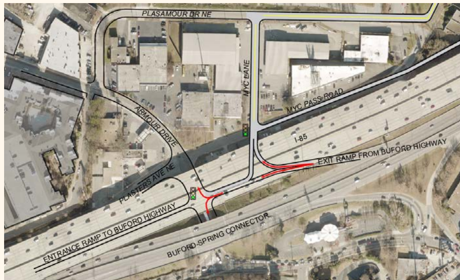
FIGURE 26. The proposed Buford Highway off ramp spur provides a direct connection from Buford Highway to the MYC development. Traffic flow with the revised configuration is shown in red.
