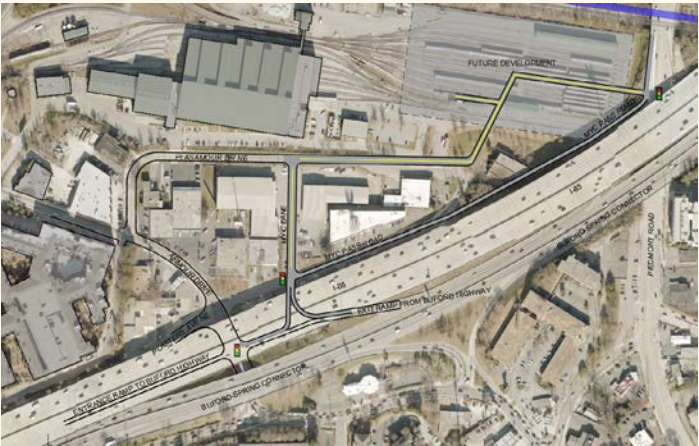
FIGURE 24. The proposed reconfiguration of the Buford Highway on and off ramps, and the local street network in Armour Ottley Yard.
